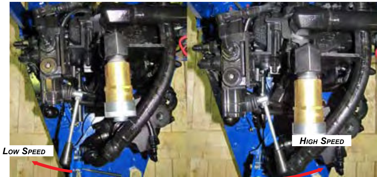
ILLUSTRATION 2.H.4: TONG MOTOR SPEED CONTROL VALVE
