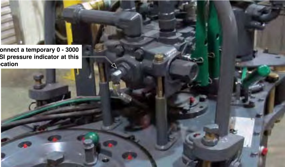
ILLUSTRATION 4.B.1: RELIEF VALVE TROUBLESHOOTING - TEMPORARY GAUGE INSTALLATION
