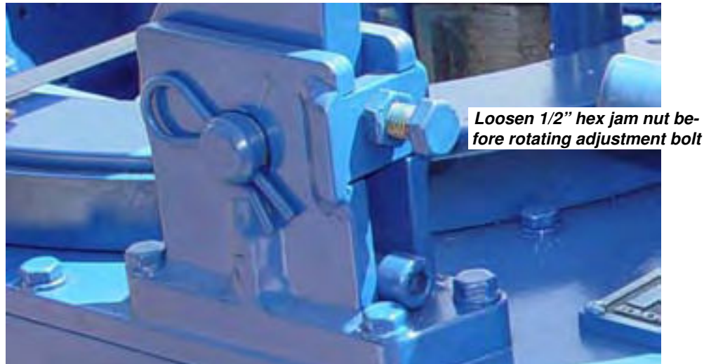
ILLUSTRATION 2.G.4: TONG LEVELING (FRONT-TO-REAR)
