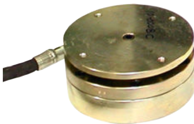
ILLUSTRATION 6.A.3: COMPRESSION LOAD CELL
