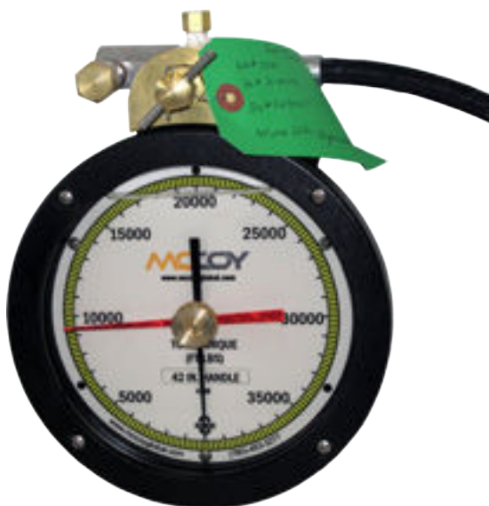
ILLUSTRATION 6.A.1: TORQUE GAUGE (FOR ILLUSTRATION PURPOSES ONLY)
