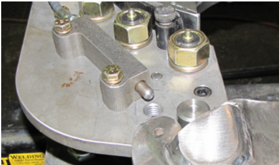
ILLUSTRATION 3.E.3: SAFETY DOOR PLUNGER ADJUSTMENT 01
