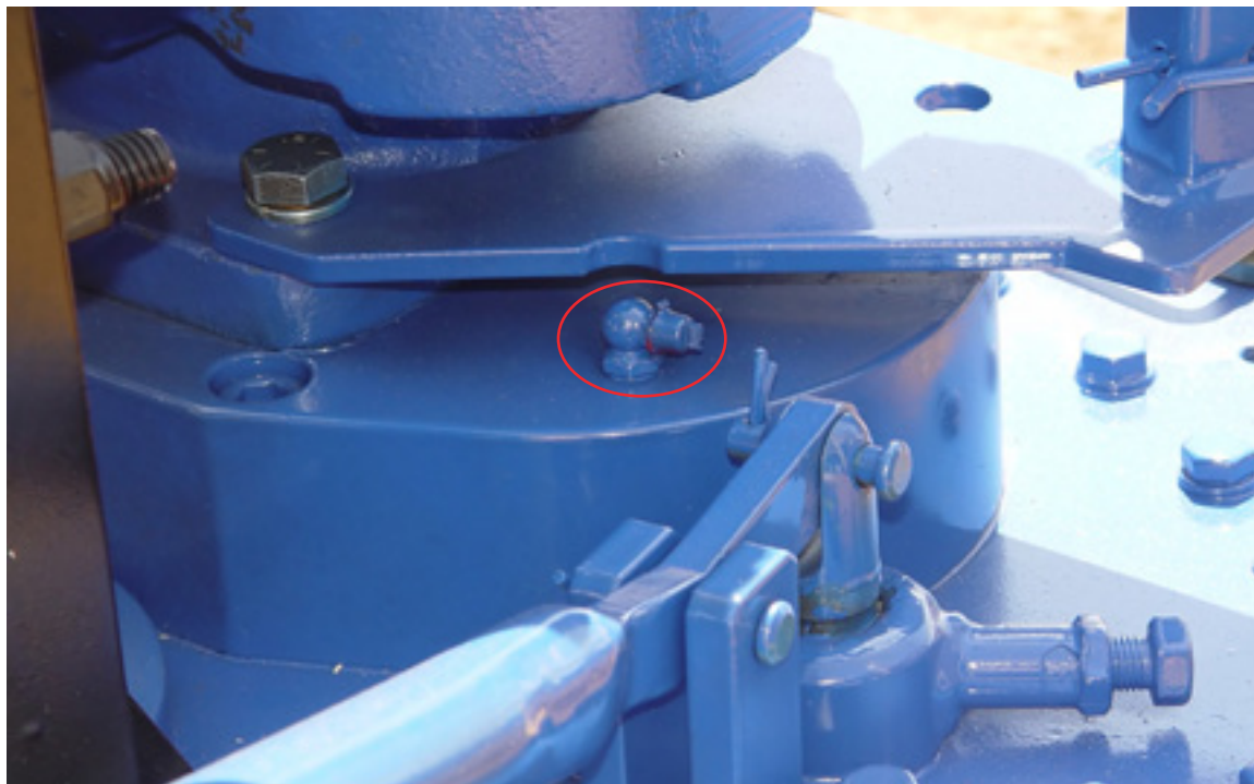
ILLUSTRATION 3.D.7: MOTOR MOUNT LUBRICATION
