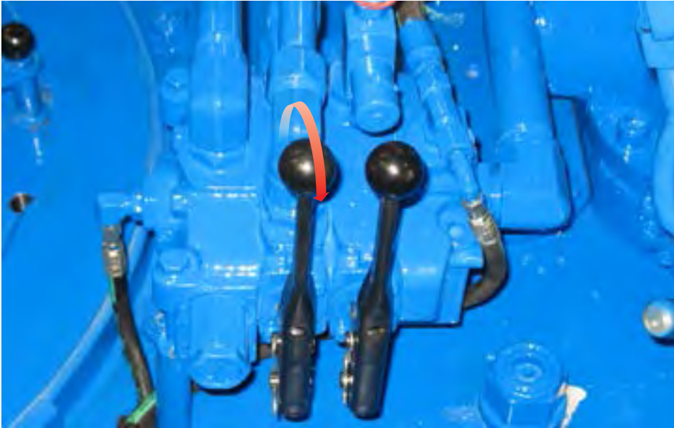
ILLUSTRATION 2.1.6: MOTOR CONTROL - RELEASING JAWS
