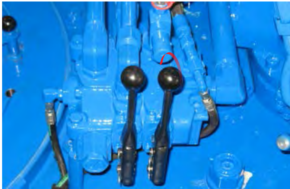
ILLUSTRATION 2.1.11: LOWERING TONG USING LIFT CYLINDER CONTROL
