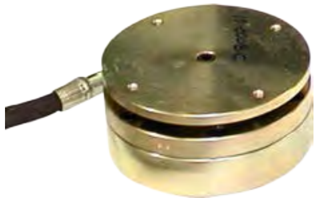
ILLUSTRATION 6.A.3: COMPRESSION LOAD CELL
