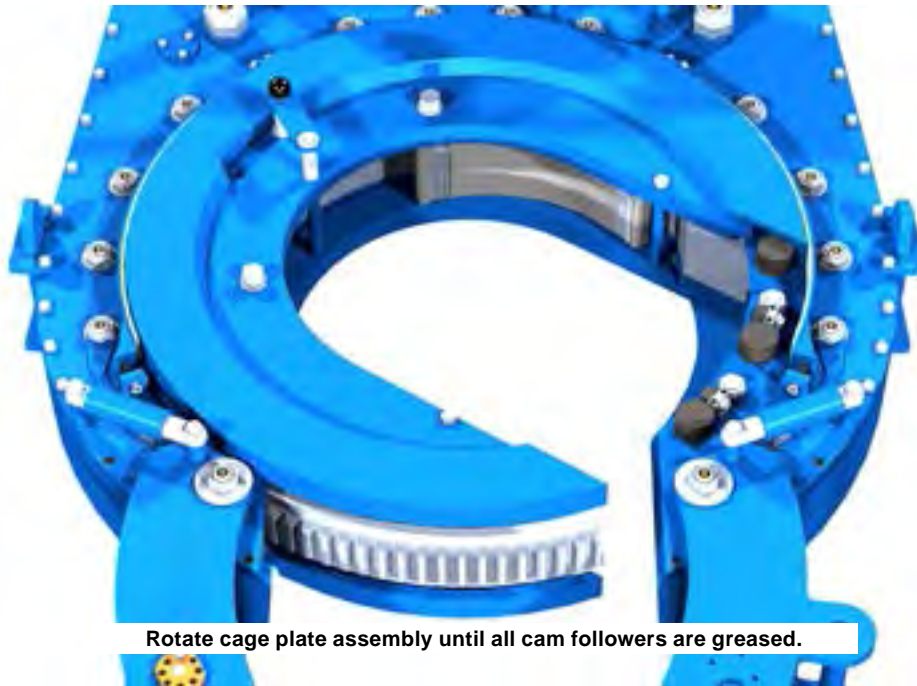
ILLUSTRATION 3.E.1: CAGE PLATE CAM FOLLOWER LUBRICATION
