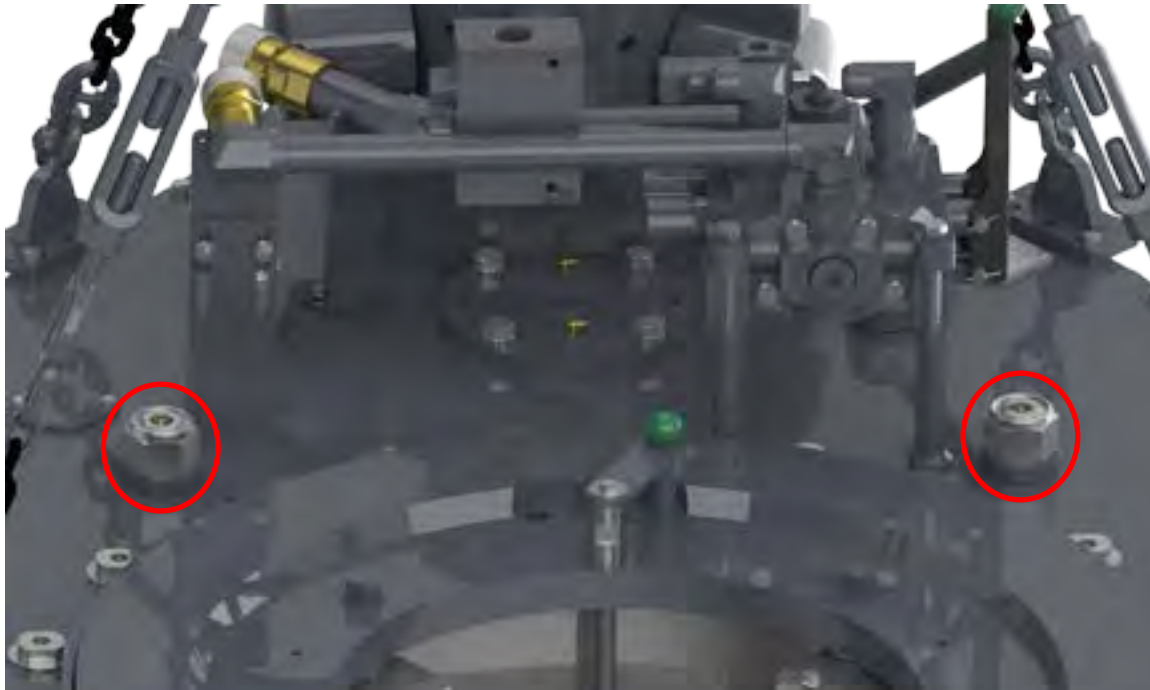
ILLUSTRATION 3.E.4: ROTARY IDLER LUBRICATION
