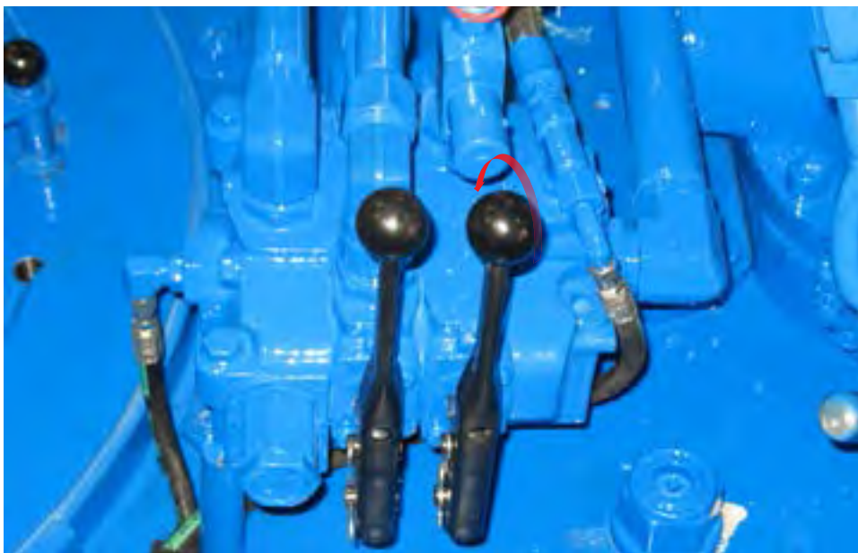
ILLUSTRATION 2.1.7: LIFT CYLINDER CONTROL - LOWER
