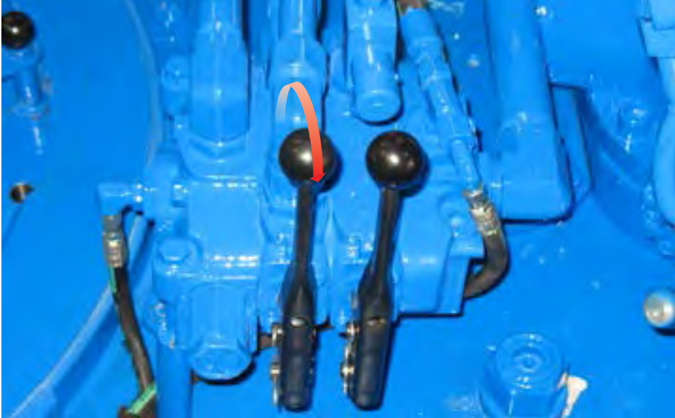
ILLUSTRATION 2.1.9: ROTATION CONTROL - BREAK-OUT
