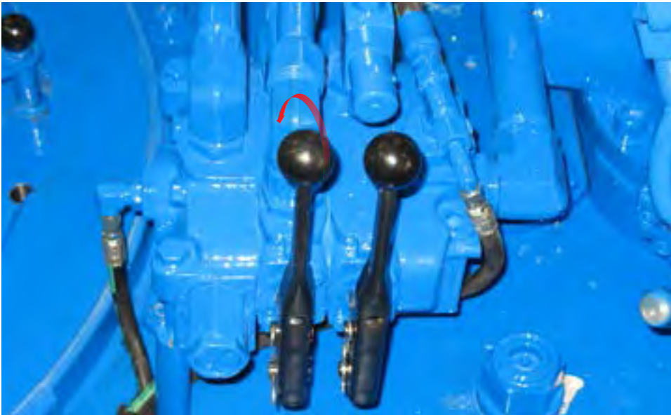
ILLUSTRATION 2.1.10: RELEASING TONG JAWS FOLLOWING BREAK-OUT & UN-THREADING
