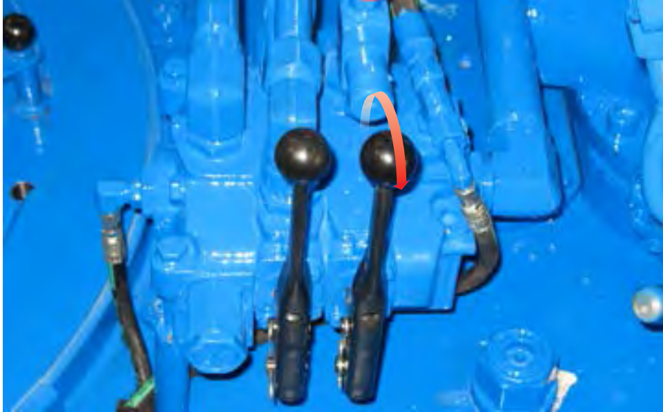
ILLUSTRATION 2.1.3: LIFT CYLINDER CONTROL - RAISE
