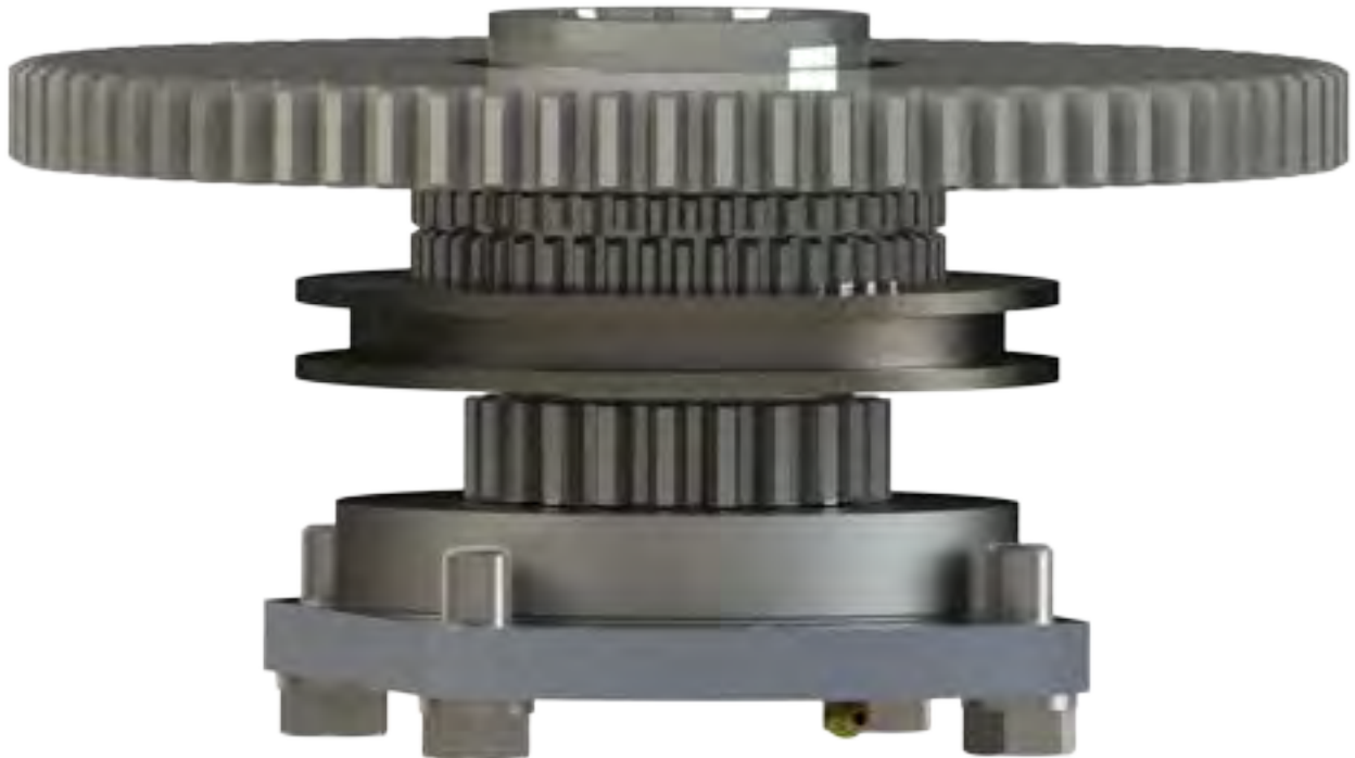
ILLUSTRATION 5.15: CLUTCH GEAR ASSEMBLY
