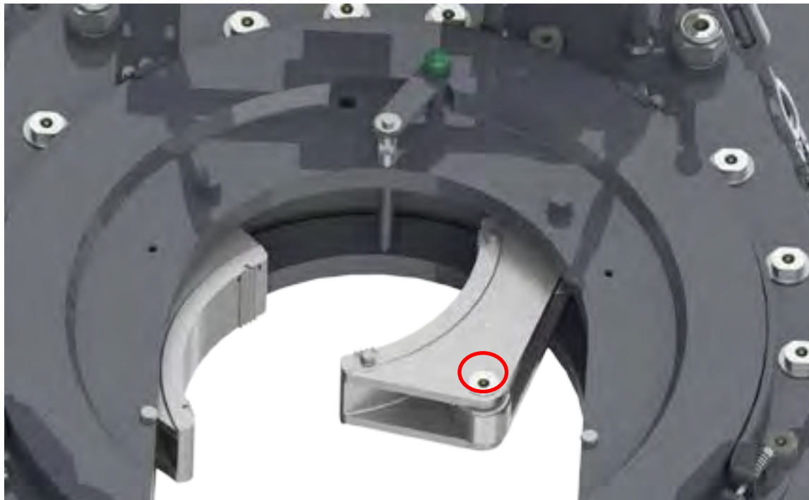
ILLUSTRATION 3.E.9: JAW ROLLER LUBRICATION
