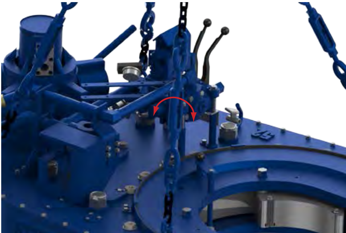
ILLUSTRATION 2.G.3: LEVELING TONG USING TURNBUCKLES
