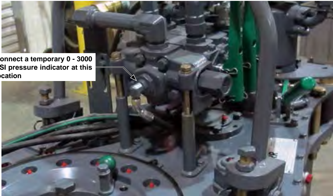
ILLUSTRATION 4.B.1: RELIEF VALVE TROUBLESHOOTING - TEMPORARY GAUGE INSTALLATION
