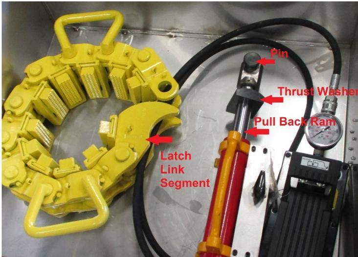
Figure 7: Air over hydraulic MP
