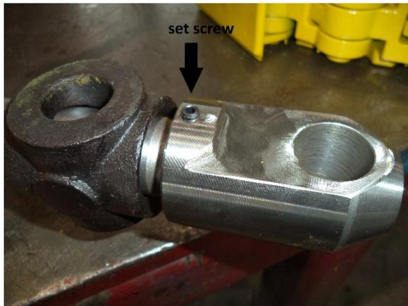
Figure 3: Set screw loosened
