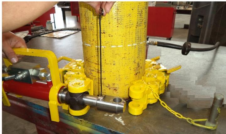
Figure 6: Tighten Set Screw
