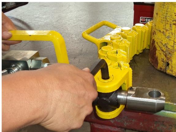
Figure 5: Tightening Pivot Block Screw
