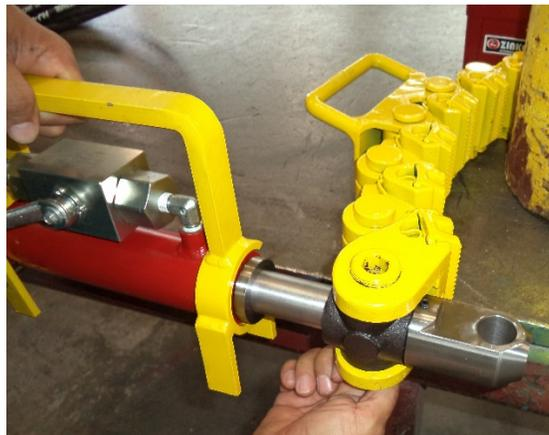
Figure 4: Pivot Block Screw
