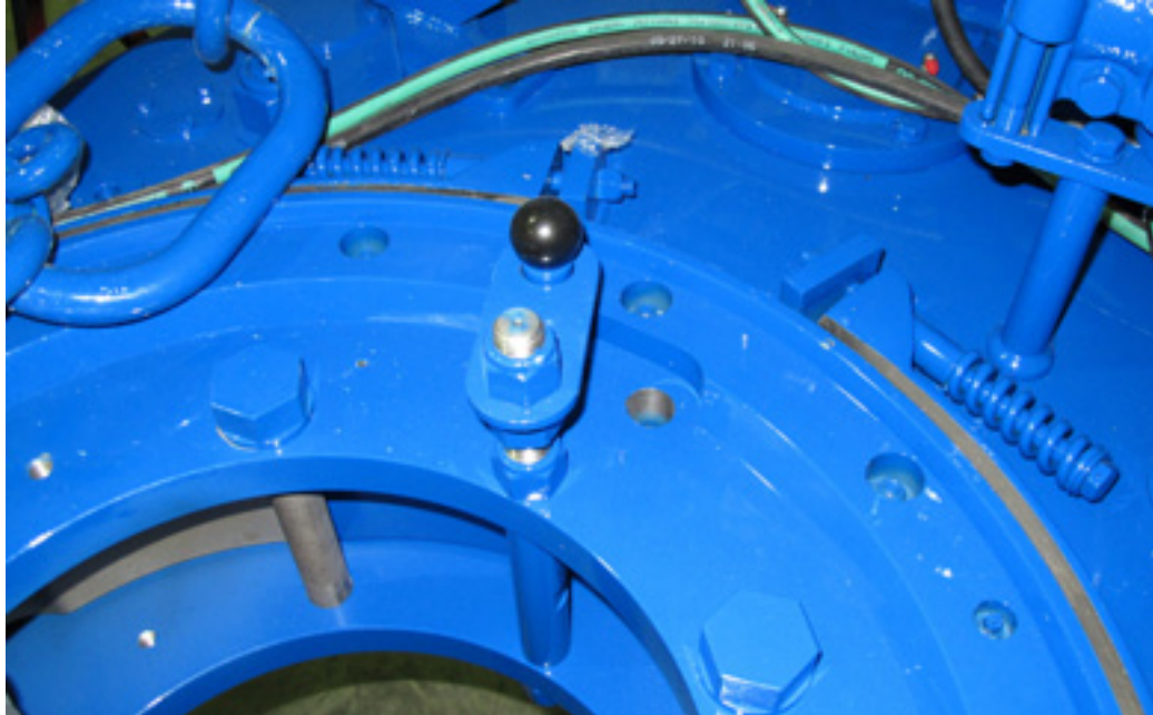
ILLUSTRATION 2.H.2: BACKING PIN SET TO "MAKE-UP" POSITION
