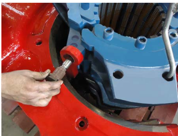
Figure 5: Slip Change – removing retainer pin
