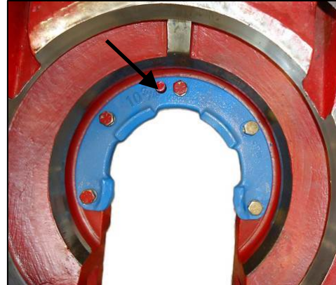
Body guide installation - use locating pin to set in place
