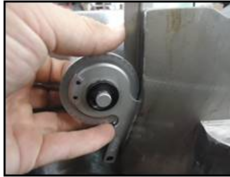
Figure 4: Measuring taper angle
