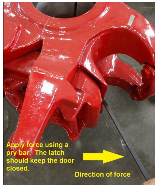
Figure 3: Pry test Instruction
