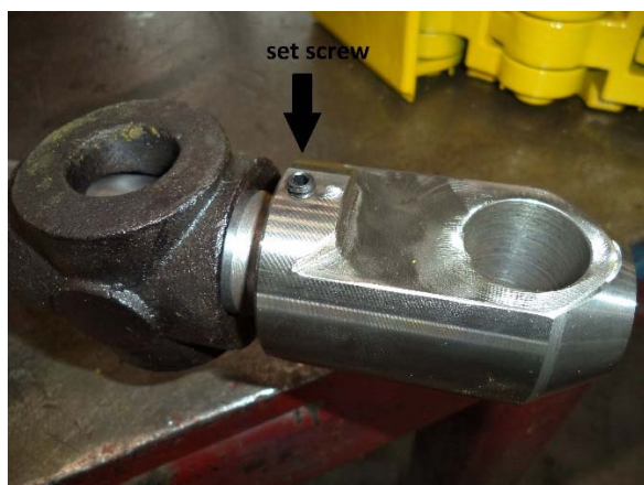
Figure 3: Set screw loosened
