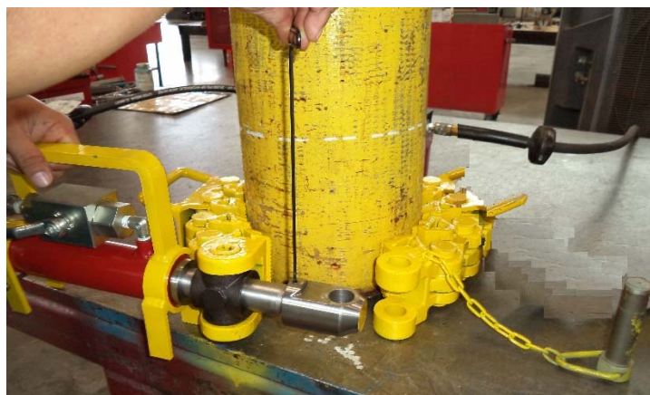
Figure 6: Tighten Set Screw
