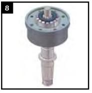
Press shaft out of bearing box.
