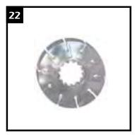
ROTOR: Normal wear results in polishing of rotor faces which does not impair motor performance.
