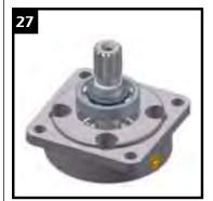
Press shaft and bearing assembly into front housing by pressing on the outer race of bearing.
