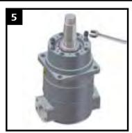
1) Two of the 3/8" bolt holes are provided with jack screw threads.
