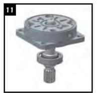
With the seal plate removed, press shaft and ball bearing out of front housing.
