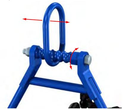
ii. Place a level lengthwise (front to back) along the tong, ensuring that it is parallel with the surface of the tong. Loosen the 3/4" jam nuts on the adjusting bolts on rigid sling brackets. Completely loosen the adjusting bolts. Turn each adjusting bolt equally until tong hangs level front-to-back. Lock adjusting bolts in place with the jam nuts.
