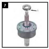
Loosen clamp screw in lock nut.
