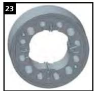
STATOR: Normal wear results in polishing of cam form which does not impair motor performances.
