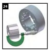
Note: Measure the rotor and stator length to the fourth decimal point and supply measurement when ordering rotor, stator, or vanes.
