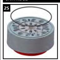
1) Reverse the procedures in steps 17, 16, 15, and 14 2) NOTE: Make sure that the radiused edge of each stator vane points to the rotor and the radiused edge of each rotor vane points to the stator.
