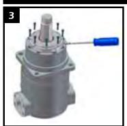
Loosen and remove 8 each 10-32 bolts.
