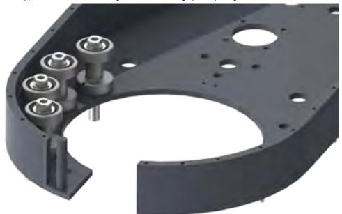
4. Install rotary gear (PN 1064-D1), making sure the backing pin slots are on the side facing up. Ensure one side is supported by the support rollers installed in Step 3, and the opening in the rotary gear is oriented toward an open support roller space as shown in the following illustration.
