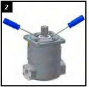
Pry out shaft seal plate with two screw drivers.
