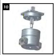
1) Remove front housing 2) Note: Two 5/16" ball checks and one main body o-ring may be dislodged and fall free.
