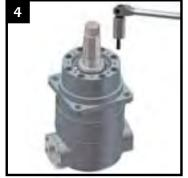
Loosen and remove 8 each 3/8" bolts with 5/16" socket head wrench.
