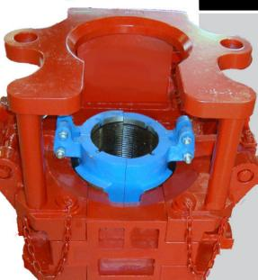
The purpose of a tubing spider is to hold the load of the tubing string as it is lowered or raised from the well.
