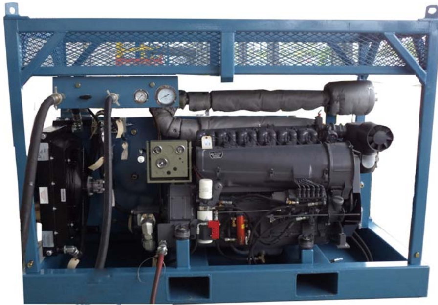
Figure 1: Power unit with air start and hoses connected
