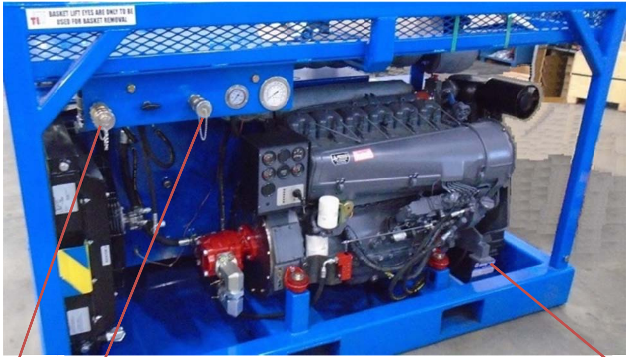
Figure 13 – Electric start naturally aspirated unit
