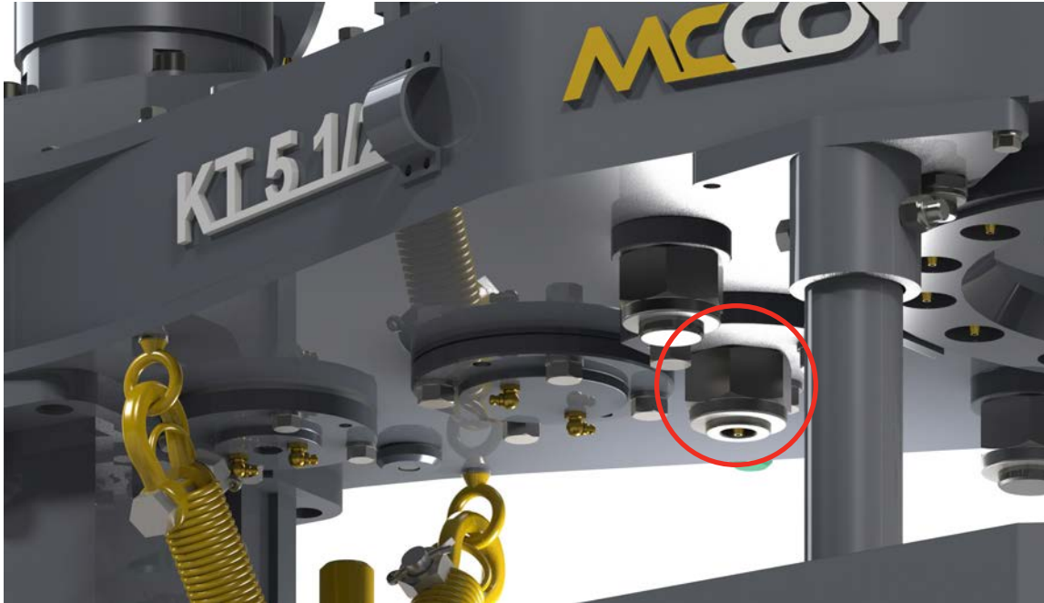
ILLUSTRATION 3.D.4: PINION IDLER BEARING LUBRICATION
