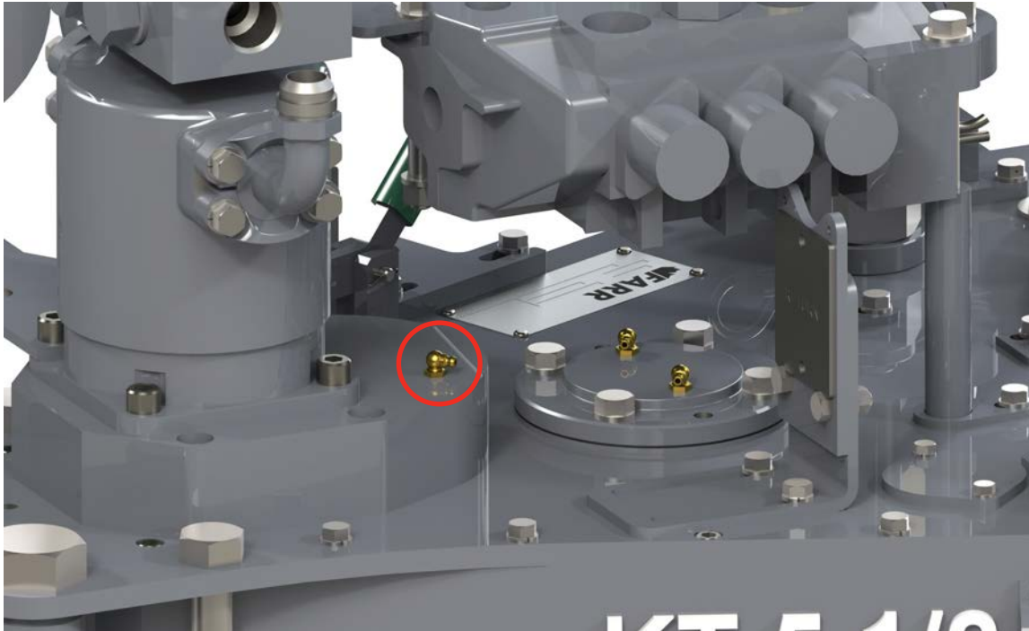
ILLUSTRATION 4.E.8: MOTOR GEAR / CLUTCH DRIVE GEAR LUBRICATION
