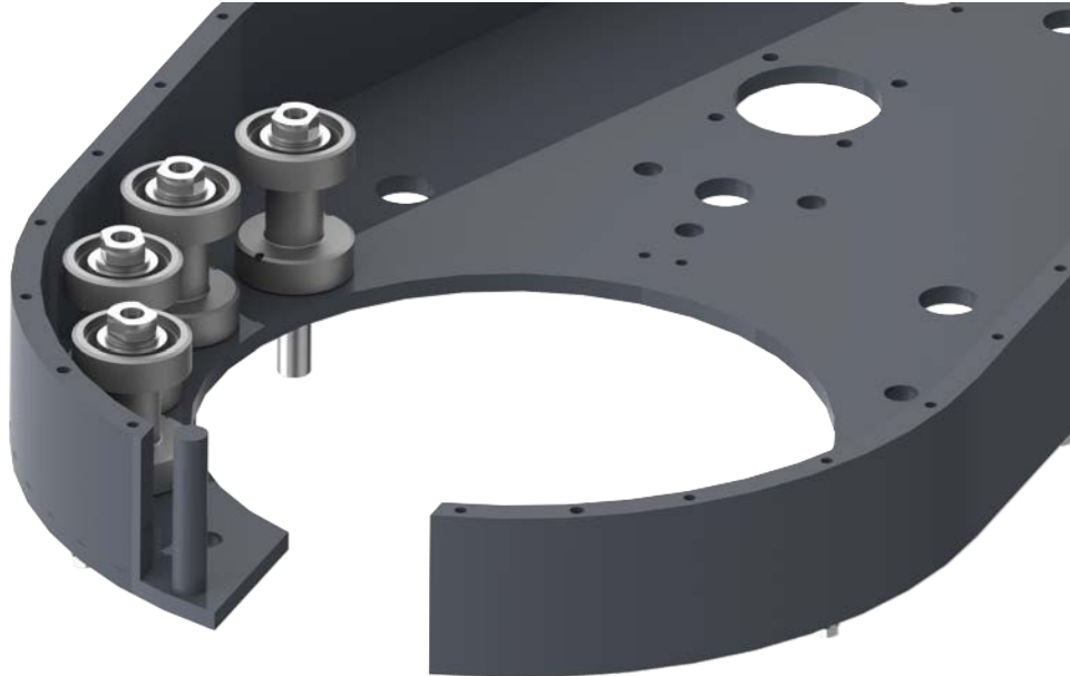
ILLUSTRATION 4.I.1: TONG ASSEMBLY - INITIAL SUPPORT ROLLER INSTALLATION
