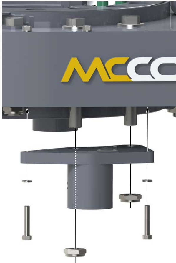
ILLUSTRATION 4.I.6: TONG ASSEMBLY - FRONT LEG MOUNT WELDMENT INSTALLATION
