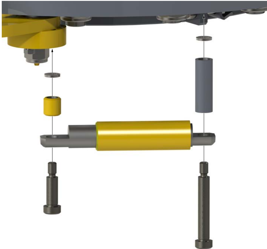
ILLUSTRATION 4.I.11: TONG ASSEMBLY - DOOR STOP SPRING CYLINDER INSTALLATION
