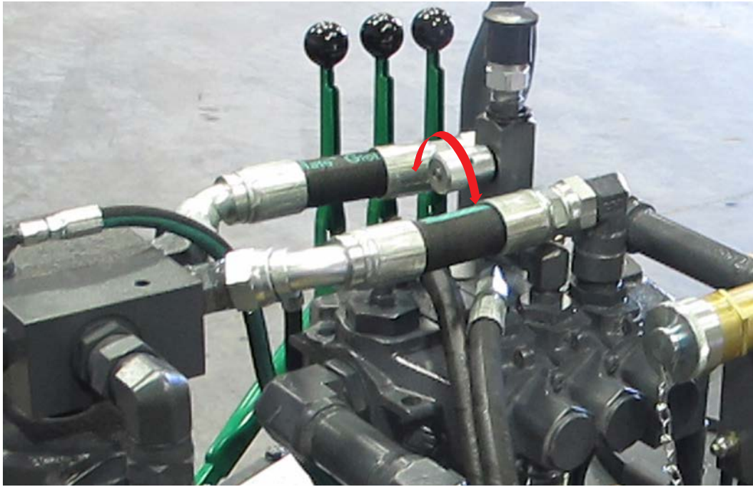
ILLUSTRATION 3.A.3: LIFT CYLINDER NEEDLE VALVE
