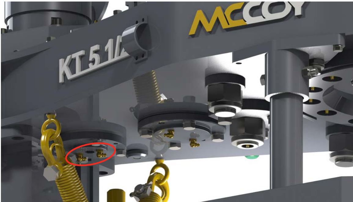
ILLUSTRATION 4.E.7: CLUTCH BEARING LUBRICATION
