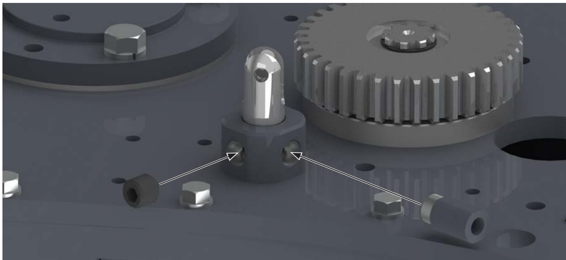
ILLUSTRATION 4.I.4: TONG ASSEMBLY - TOP SHIFTER BUSHING INSTALLATION
