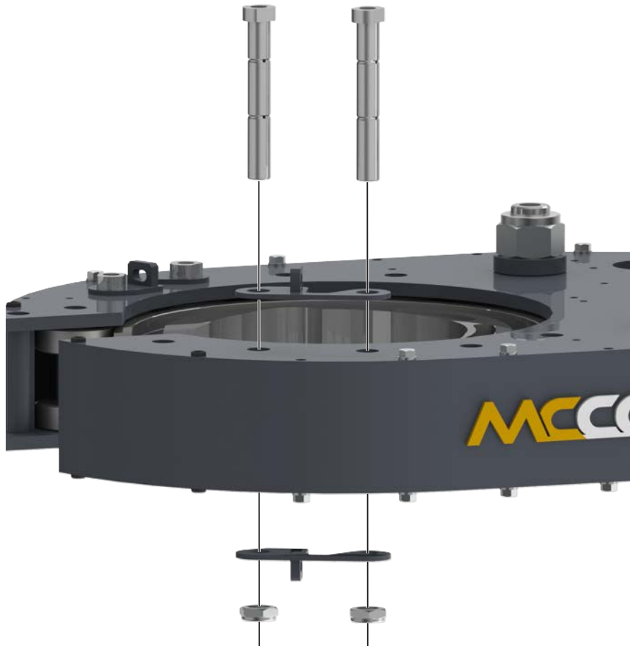
ILLUSTRATION 4.I.5: TONG ASSEMBLY - BRAKE BAND WELDMENT INSTALLATION
