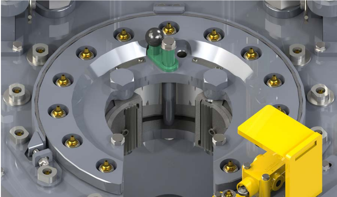
ILLUSTRATION 3.B.2: BACKING PIN CONFIGURED FOR "MAKE-UP" OPERATIONS
