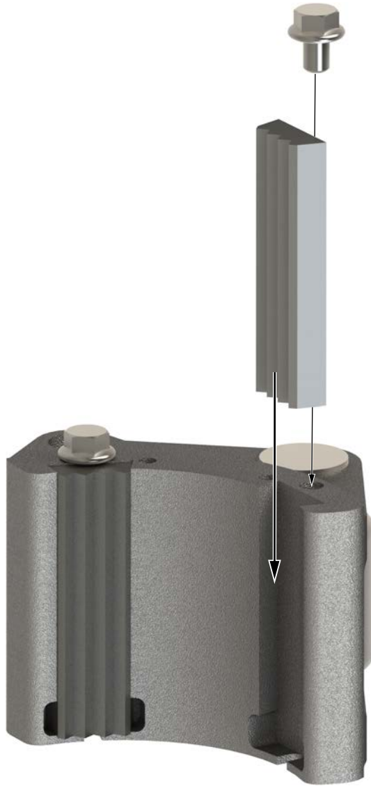
ILLUSTRATION 2.F.2: KT5500 STANDARD JAW DIE REMOVAL
