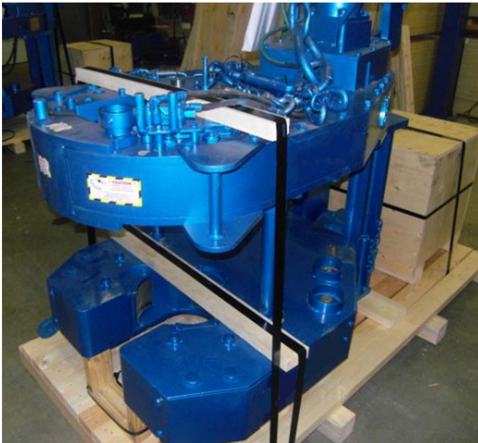
ILLUSTRATION 4.M.4: SHIPPING INSTRUCTIONS - STRAPPING EQUIPMENT TO PALLET
