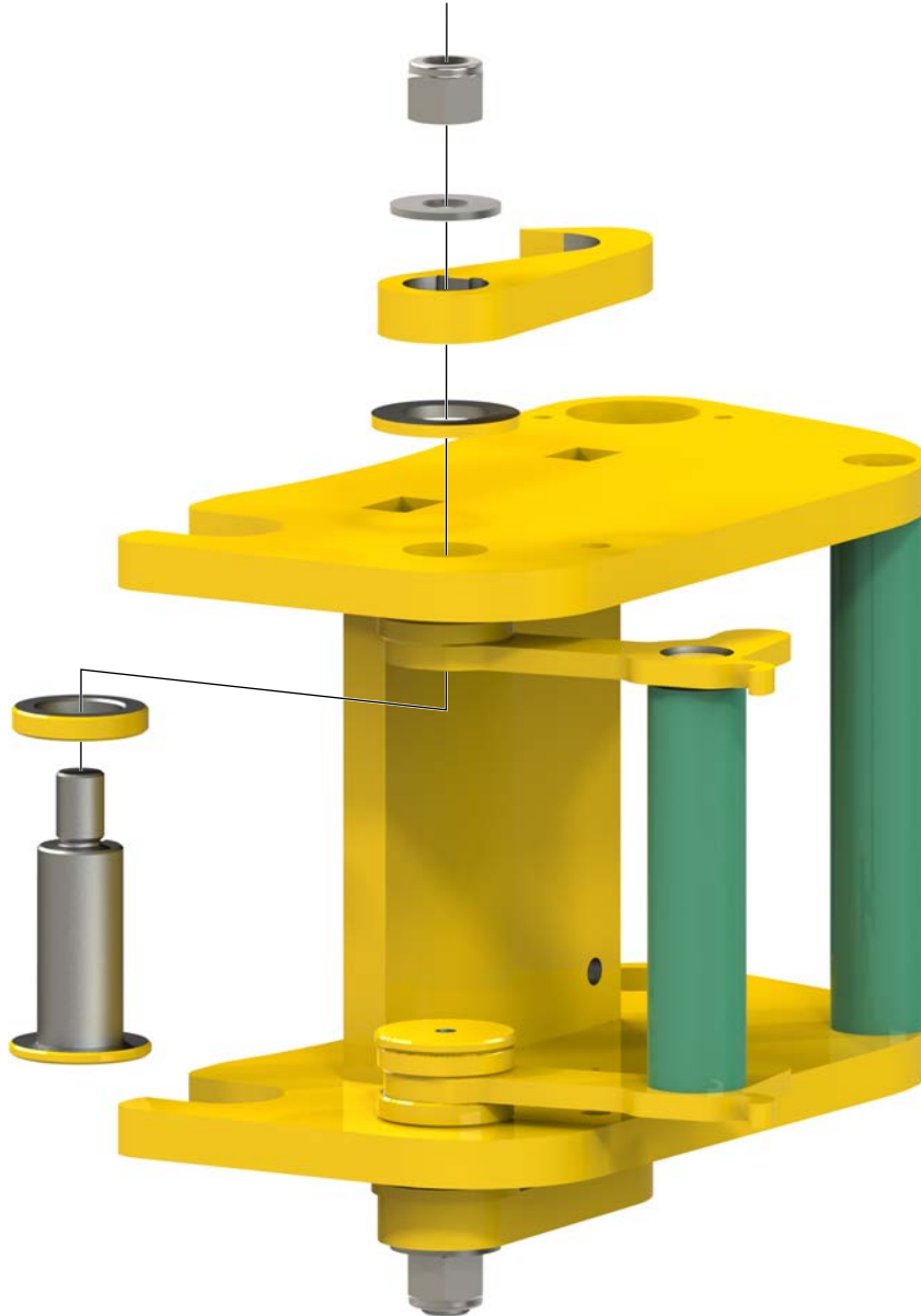
ILLUSTRATION 4.I.8: TONG ASSEMBLY - LATCH INSTALLATION 02
