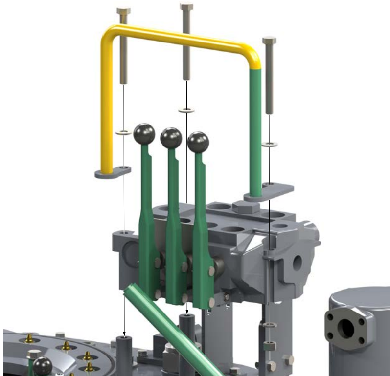
ILLUSTRATION 4.I.12: TONG ASSEMBLY - VALVE ASSEMBLY INSTALLATION
