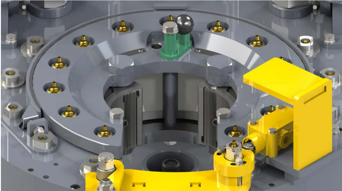
ILLUSTRATION 3.B.4: BACKING PIN CONFIGURED FOR “MAKE-UP” OPERATIONS
