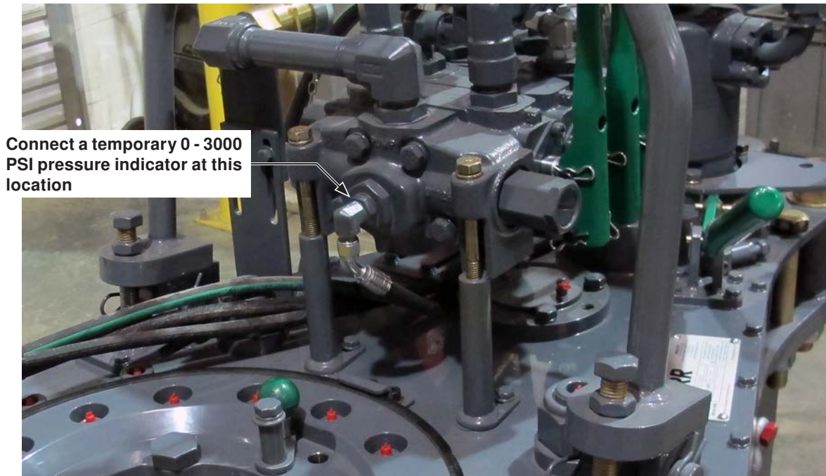
ILLUSTRATION 5.B.1: RELIEF VALVE TROUBLESHOOTING - TEMPORARY GAUGE INSTALLATION
