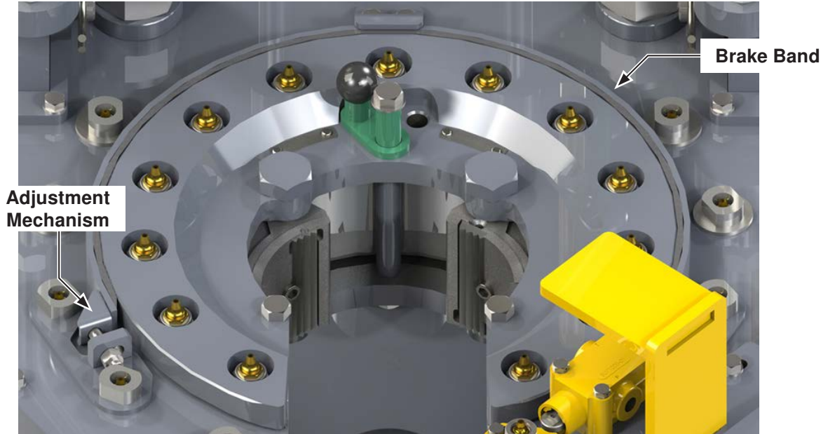
ILLUSTRATION 4.F.1: BRAKE BAND ADJUSTMENT
