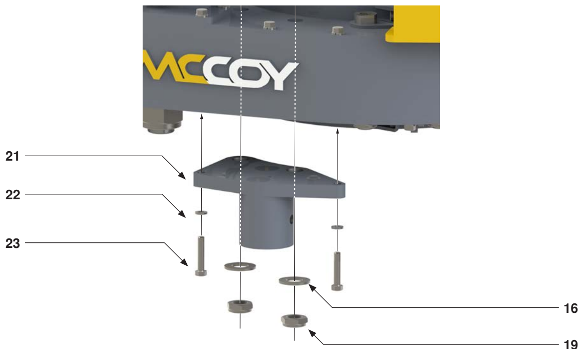
ILLUSTRATION 6.39: FRONT LEG WELDMENT INSTALLATION
