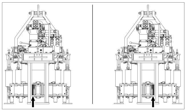
**Illustration 3.6.2: Make Up Load Cell Configuration**
