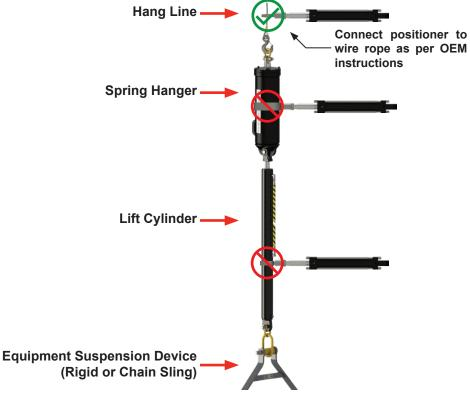
Illustration 3.2.1: Correct Installation of Positioning System
