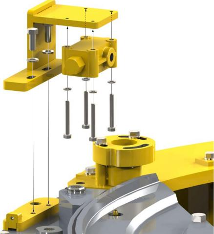
Illustration 5.9.14: Rotation Interlock Switch Installation
