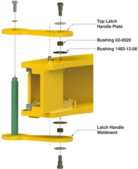
Illustration 5.9.8: Tong Assembly - Door Latch Handle Installation
