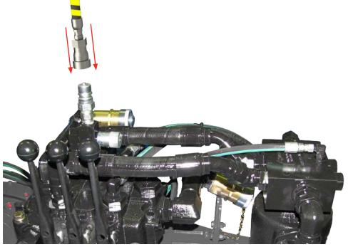
Illustration 3.2.2: Lift Cylinder Hydraulic Connection
