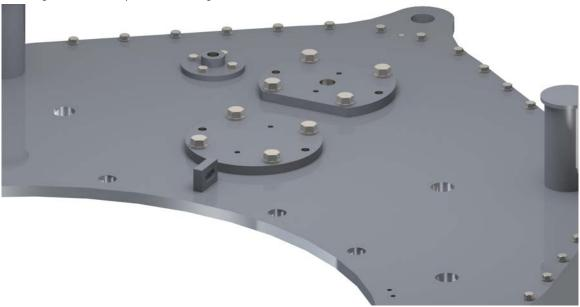
Illustration 5.9.1: Tong Assembly - Lower Bearing Cap Installation
