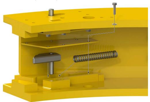
Illustration 5.9.7: Tong Assembly - Latch Claw & Spring Installation
