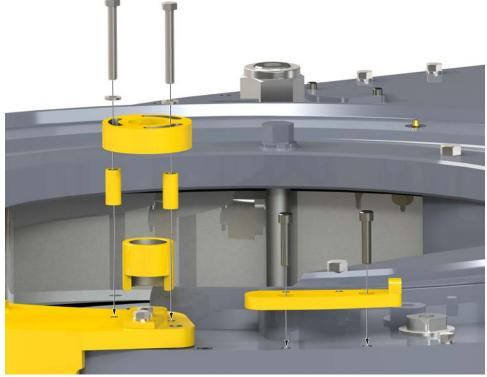
Illustration 5.9.12: Rotation Interlock Component Installation
