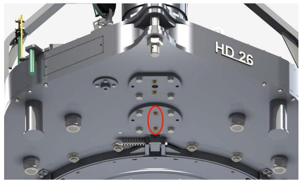
Illustration 5.5.6: Pinion Bearing Lubrication (Bottom Plate)
