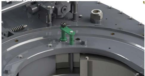
Illustration 4.1.2: Backing Pin Set To "Make-up" Position
