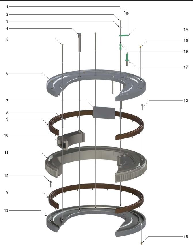
Illustration 7.19: Cage Plate Assembly Exploded
