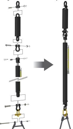
Illustration 3.2.1: Lift Cylinder & Spring Hanger Installation
