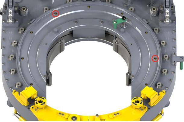
Illustration 5.5.1: Cage Plate Guide Ring Lubrication
