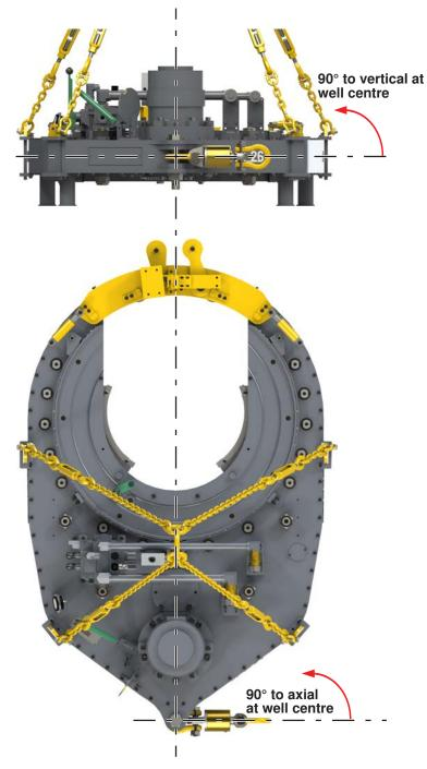
Illustration 3.5.1: Tong Suspension and Load Cell Orientation
