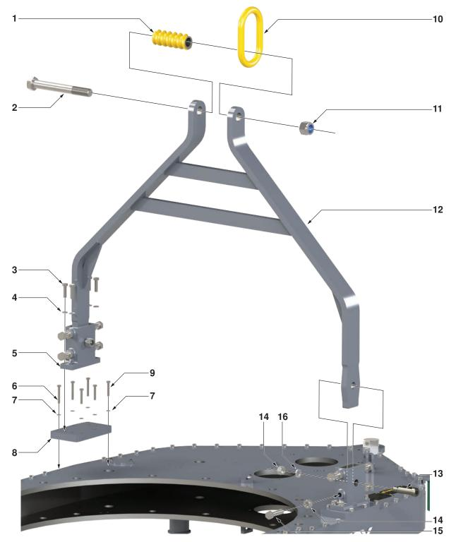
Illustration 7.33: Rigid Sling Assembly Exploded
