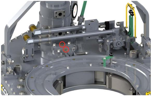
Illustration 5.5.5: Pinion Bearing Lubrication (Top Plate)
