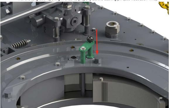
Illustration 4.1.3: Setting Backing Pin To "Break-Out" Position
