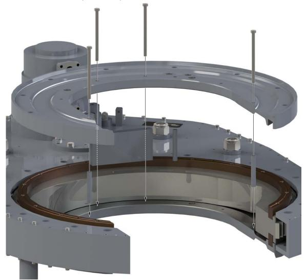
Illustration 5.9.6: Tong Assembly - Cage Plate Assembly
