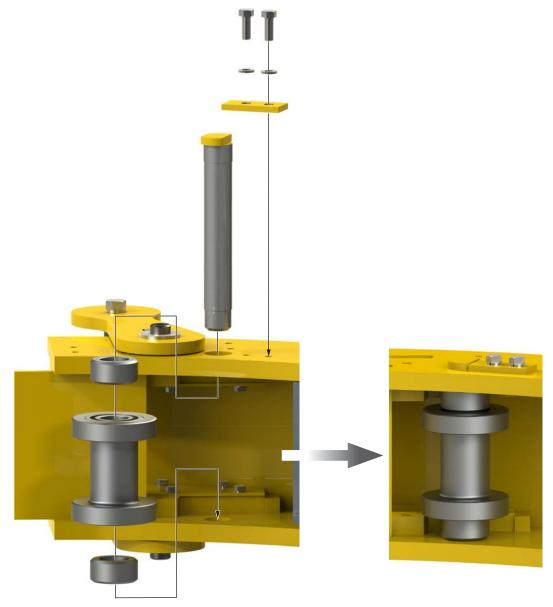
Illustration 5.9.10: Tong Assembly - Door Roller Installation
