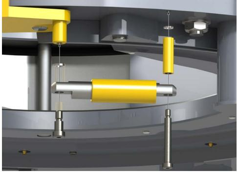
Illustration 5.9.13: Door Spring Stop Cylinder Installation
