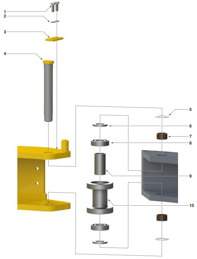
Illustration 7.9: Support Roller (Door Pivot) Exploded
