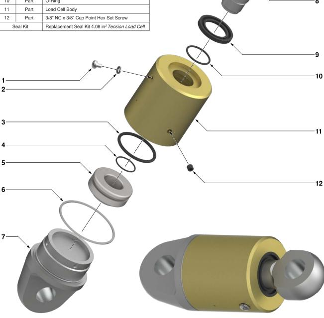
Illustration 8.0.3: Tension Load Cell Exploded
