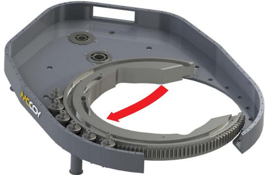
Illustration 5.9.3: Tong Assembly - Rotary Gear Installation
