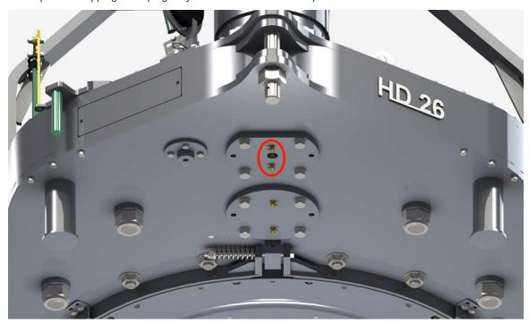
Illustration 5.5.7: Clutch Bearing Lubrication
