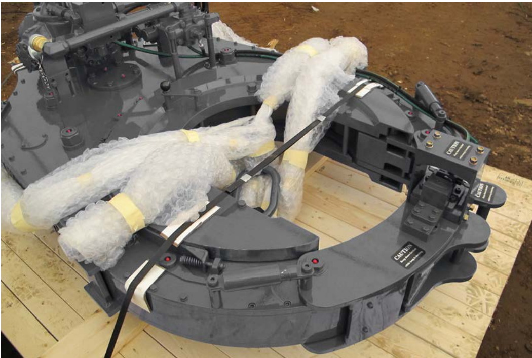
Illustration 5.12.2: Shipping Instructions - Strapping to Pallet
