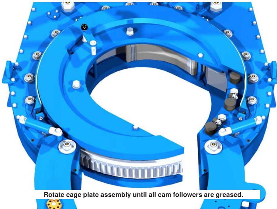
ILLUSTRATION 3.E.1: CAGE PLATE CAM FOLLOWER LUBRICATION
