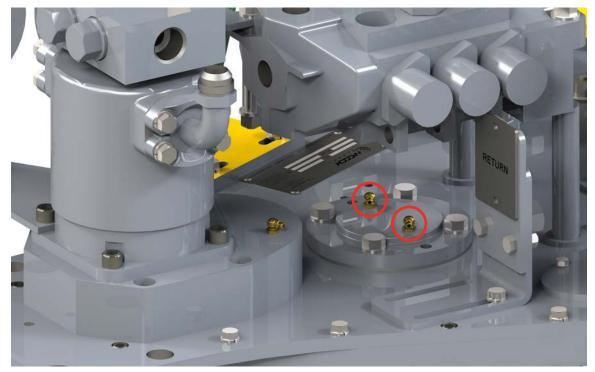
Illustration 5.5.5: Pinion Bearing Lubrication
