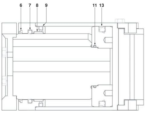
Illustration 7.45: 1403-00-00B 5-1/2" Clincher Cylinder Exploded
