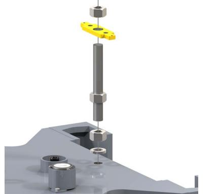
Illustration 5.9.11: Tong Assembly - Rear Backup Spring Support Bracket Installation
