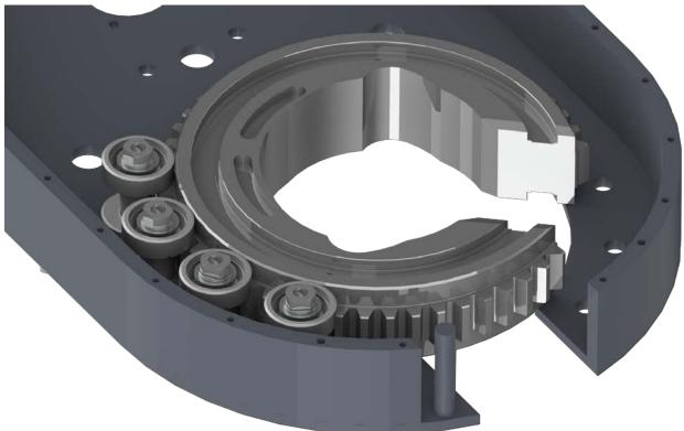
Illustration 5.9.2: Tong Assembly - Rotary Gear Installation
