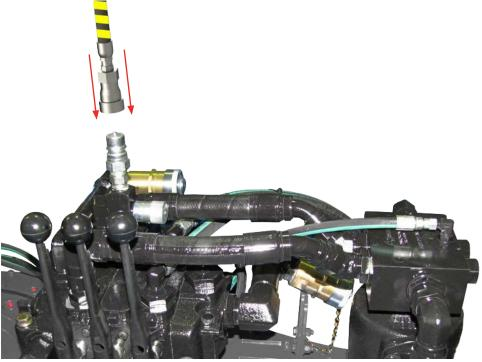
Illustration 3.2.2: Lift Cylinder Hydraulic Connection
