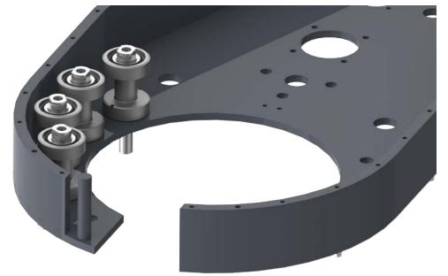
Illustration 5.9.1: Tong Assembly - Initial Support Roller Installation
