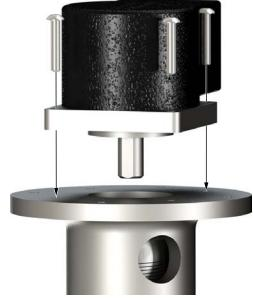
Illustration 8.1.3: Securing Encoder To Encoder Mount
