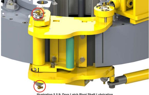
Illustration 5.5.9: Door Latch Pivot Shaft Lubrication
