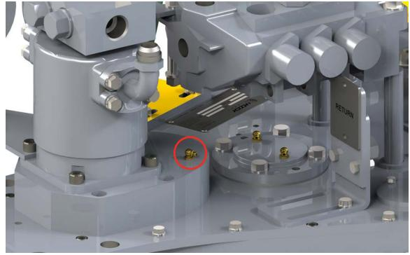
Illustration 5.5.7: Motor Gear / Clutch Drive Gear Lubrication
