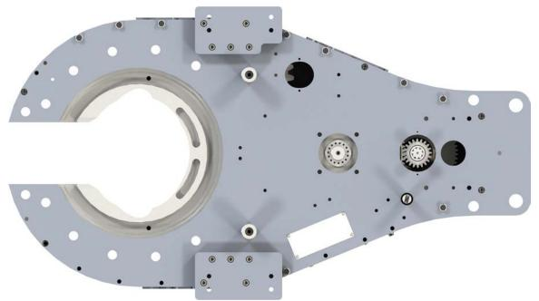
Illustration 5.9.4: Tong Assembly - Top Plate Fastener Installation
