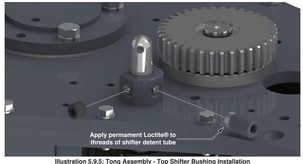
36. Insert the detent ball (PN 02-0018) through the end of the detent tube attached to the top shifter bushing, followed
