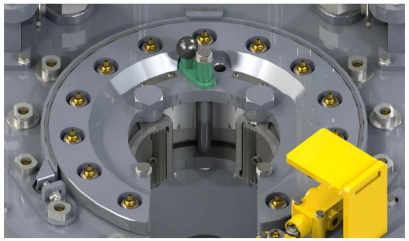
Illustration 4.1.2: Setting Backing Pin To "Make-up" Position
