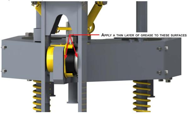
Illustration 5.5.13: Load Cell Lubrication
