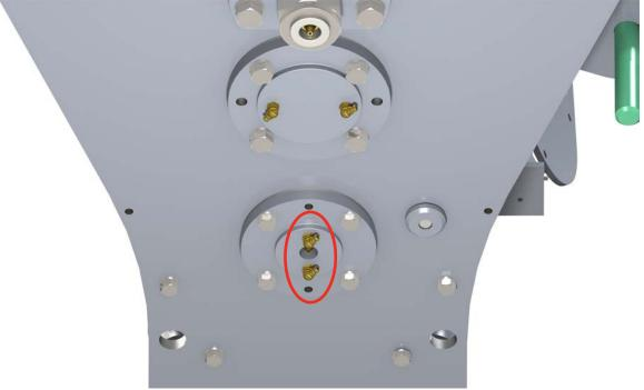
Illustration 5.5.6: Clutch Bearing Lubrication
