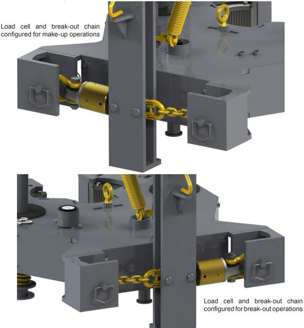
Illustration 3.5.6: Tension Load Cell Configuration
