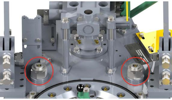
Illustration 5.5.3: Rotary Idler Bearing Lubrication
