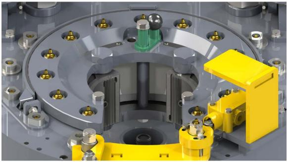
Illustration 4.1.3: Backing Pin Set To "Break-Out" Position
