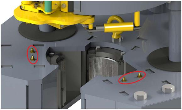
Illustration 5.5.12: CLINCHER© Cylinder Lubrication
