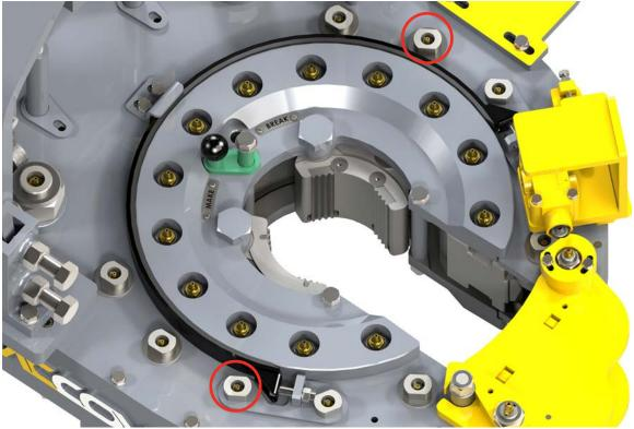
Illustration 5.5.2: Support Roller Bearing Lubrication
