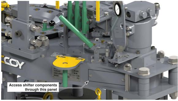
Illustration 5.5.8: Shifting Shaft Lubrication
