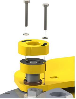
Illustration 5.9.8: Tong Assembly - Door Switch Cam Installation
