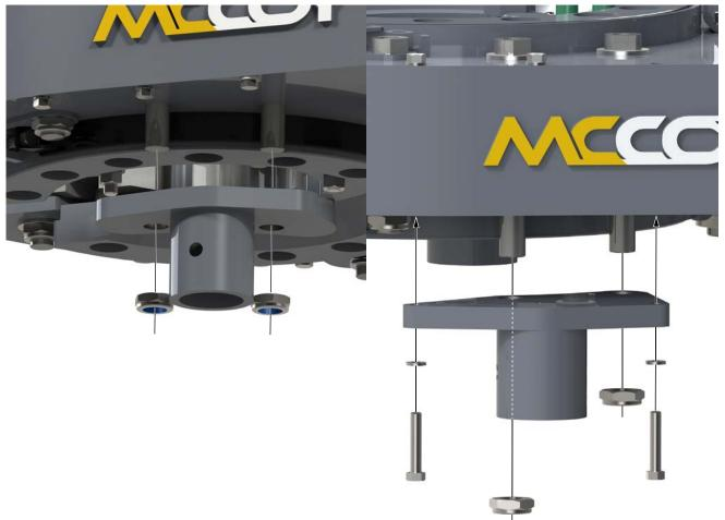
Illustration 5.9.7: Tong Assembly - Front Leg Mount Weldment Installation
