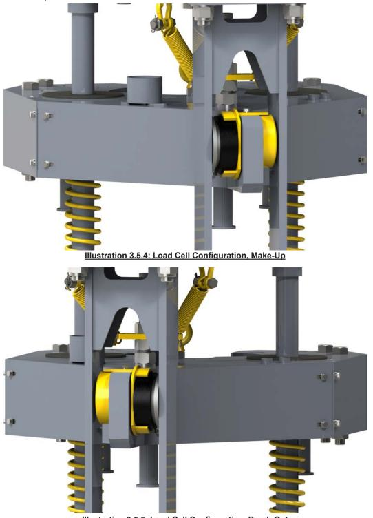
Illustration 3.5.5: Load Cell Configuration, Break-Out
