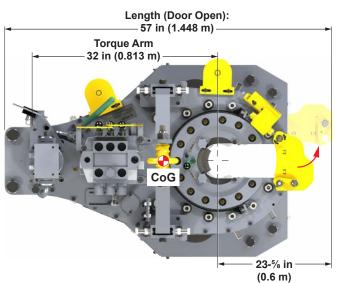
Center of gravity shown on these assembly drawings does not include installed jaws.
