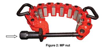
With the clamp installed, the spring loaded tapered inserts are designed to firmly grip and wedge against the tubular as the load increases or as the tubular slips down. As the load increases, the spring tension and taper will result in a tighter grip that prevents further travel.
