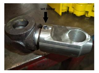
Figure 3: Set screw loosened
