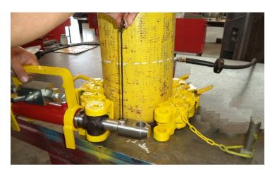
Figure 6: Tighten Set Screw
