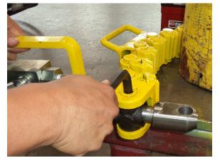
Figure 5: Tightening Pivot Block Screw
