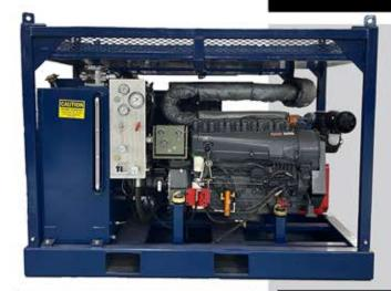
Deutz 6 cylinder, Diesel powered with Air Start, skid mounted hydraulic power unit.
